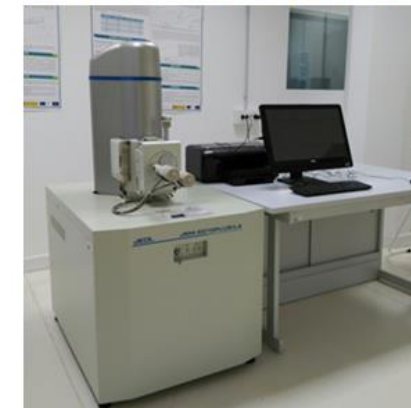
SEM-EDS JEOL 6010PLUS/LA 20kV
